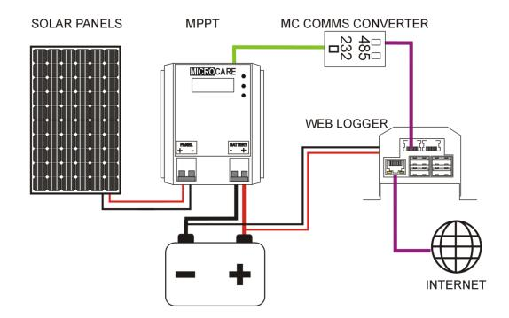
In this configuration, a single Microcare MPPT is connected to a MC COMS converter. The MC COMS converter is then connected to the MC COMS port of the Web-Logger. The LAN or Ethernet port of the Web-Logger is then connected to an Internet enabled router.
