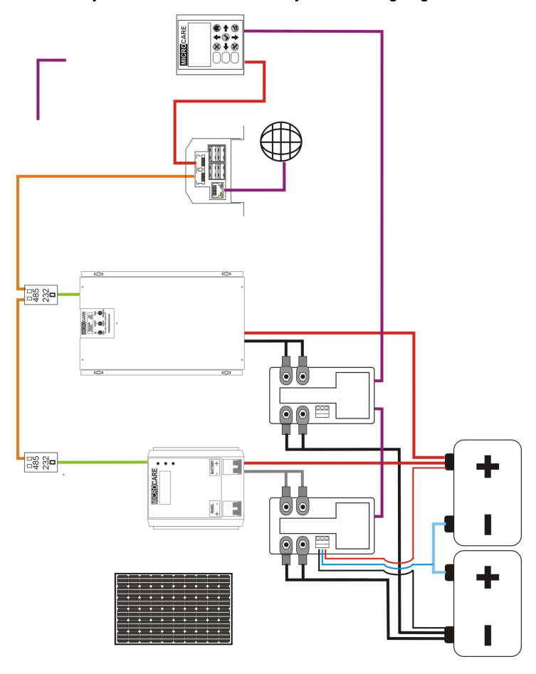
In this configuration the Web-Logger, Battery Monitor and RS232-485 converters all connect in series creating the Microcare communications network.
