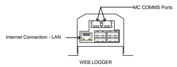
The Web-Loggers' power is supplied by the connected battery bank. Supply voltage to not exceed 70V DC!
