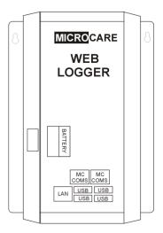
Plug the Ethernet cable into the silver Ethernet port of the Web-Logger (bottom row on the left hand side) and plug the other end of the Ethernet cable into your internet router. The Web-Logger uses DHCP to obtain a network connection automatically. The green and orange network LEDs will flash indicating a network connection to the router.
